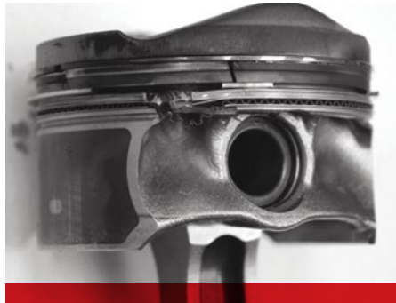
Low Speed Pre-Ignition (LSPI) is a relatively new phenomenon in gasoline/petrol piston failures. Seen here are the results of an LSPI failure in a 3.5 liter Ecoboost.
